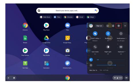
Step 3. Open the status bar in the lower-right corner of the screen and select <sup>(a)</sup>.
